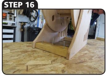
PREDRILL THE 3" SCREWS BEFORE MOUNTING TO WALL
