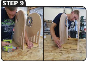
PLACE REMAINING 2x4s INTO POCKETS AND SCREW 2" SCREWS INTO PREDRILLED HOLES
