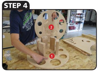
TAKE INNER WHEEL 2, ALIGN WITH 2x4s, AND FIT INTO PLACE
