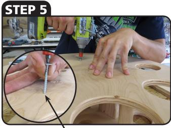
FIND THE 5 PREDRILLED HOLES AND DRILL 2" WOOD SCREWS INTO 2x4s
