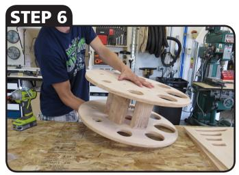
PLACE ONE HAND ON TOP AND ON THE UNDER SIDE OF THE INNER WHEELS. CAREFULLY FLIP TO THE OTHER SIDE AND REPEAT STEP 5
