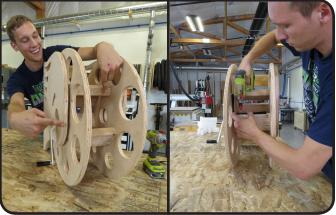
LOCATE THE LARGE SPACE BETWEEN THE 2x4s AND ATTACH 10" FASTWRAP ON THE HANDLE SIDE
