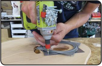
THEN ATTACH WITH MINI POWERHEAD SCREWS
