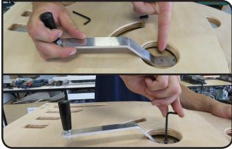
ALIGN HANDLE WITH THE PREDRILLED HOLES AND SECURE WITH 1/4"-20x3/4"BOLTS
