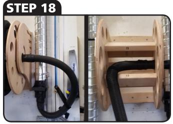
ATTACH VACUUM TO OUTSIDE OF THE SUPER REEL AND ATTACH HOSE TO INSIDE. SECURE HOSE WITH FASTWRAP AND REWIND YOUR HOSE!
