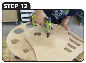
SECURE ROLLER BEARING WITH MINI POWERHEAD SCREWS, FLIP SUPER REEL TO OTHER SIDE, AND REPEAT STEP 11
