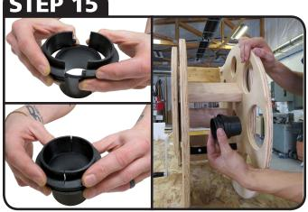
ASSEMBLE AND PLACE THE VACUUM SWIVEL CUFF INTO HOLE OPPOSITE THE HANDLE \*Note: Longer side of the swivel cuff facing out.
