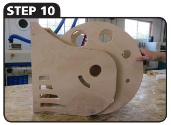
ROLL WHEEL INTO OUTER PANEL AND ALGIN WITH CENTER HOLES
