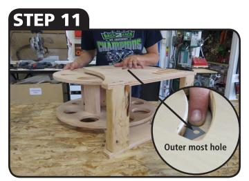
FLIP THE SUPER REEL ON ITS SIDE AND ALIGN EACH CORNER OF ROLLER BEARING WITH PREDRILLED HOLES
